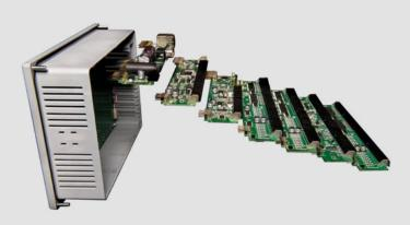
The boards can be plugged into one of the 5/7/8 slots available without any constraints. The system is equipped with a self-detecting and self-addressing resources mechanism, that allows an easy, fast and flexible installation.
